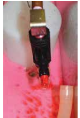
Step 4: Then we will replace it with a red tip. Screw it in and replace the hose.
