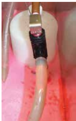
Step 1: The first thing you're going to do is take the pick-up tube off. Which on most Hydrominders is just a matter of pulling.
